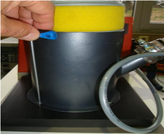
Loosen the fixing screws and open the funnel.
