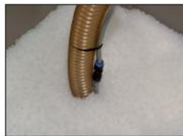
Correct: The lance is pressed deeply into the granules
