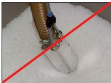
Wrong: The lance is positioned on top of the granules
