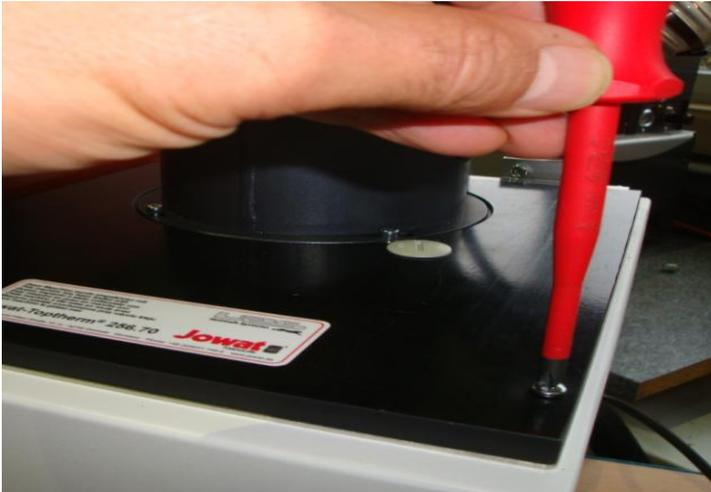
Loosen the fixing screws and open the funnel.
