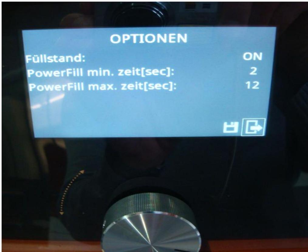
The filling time is set at the factory to a minimum of 2 sec and a maximum of 12 sec.
