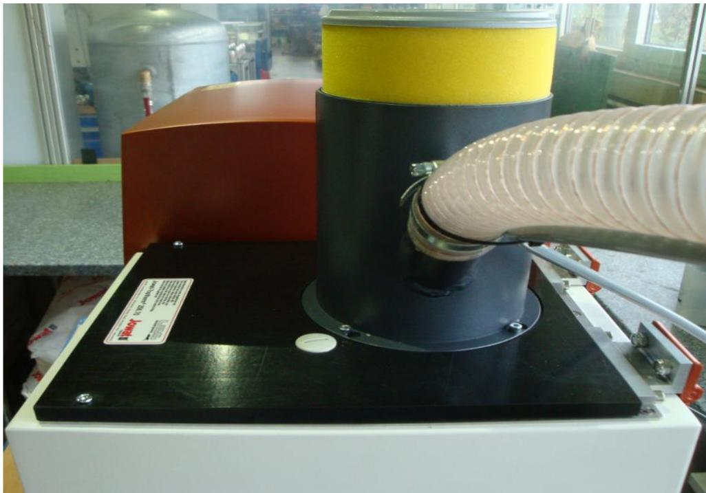
**Attach the delivery hose to the filler neck using the hose clamp.**
